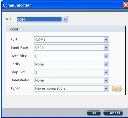
Figure 19: Remote GSM connection set up
